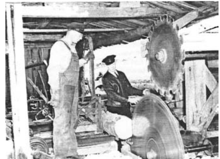
Ogden sawmill - Verlon (in dark coat) runs the carriage past the spinning saw, while his brother Earl sets the lumber thickness
